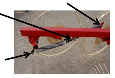
**Adjusting the wings:** Raise or lower the clevis hitch in the tongue to level the main arms. The retaining bolt for the wheel arms should be close to the center of the slotted hole in the main arm front to rear. If they are all high or low adjust the cylinder clevis as explained on page 9. If they are high in the front and low in the rear or vice versa then raise or lower tongue to make them all the same. Then adjust the cylinder clevis to bring them to the center.
