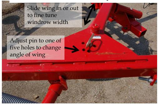
Adjust the wing angle and slide tube extensions (HCI only) to get the raking width and windrow width desired. Adjust the rake wheel angle first. **Remember the rake wheel angle should be adjusted according to crop conditions.** For heavy crop you want narrower raking width with less angle on rake wheels and for light crop you want wider raking width with more angle on the rake wheels. Then fine tune the windrow width by sliding the wings in or out (HCI-RCI only).
