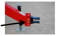
The main arms must be close to level and the wheel arm retaining bolts close to the center of the slotted holes for the wheel arms to float properly!
