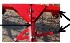
HINT: To slide wing in or out on RH wing pull handle with right hand and push main arm out with left hand simultaneously. On LH wing pull handle with left hand and push main arm out with right hand simultaneously.
